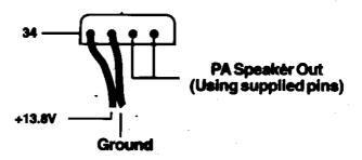
Supplied Power Cord - Connect supplied power cord to the keyed connector.
